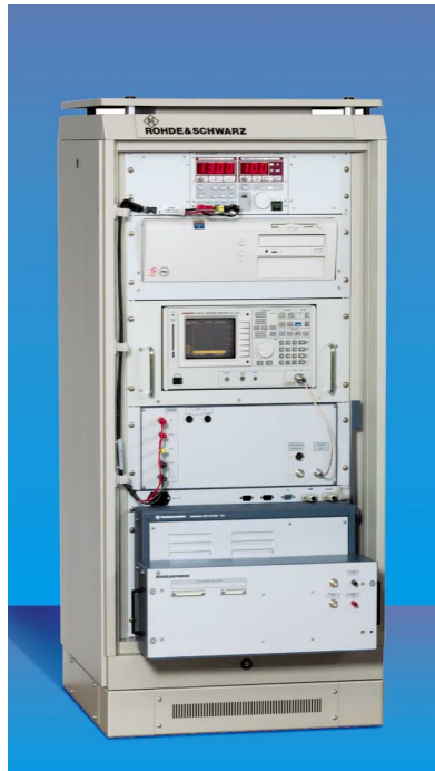
FIG 3 Repair station for receivers based on Universal Test System TSU Photo 43 124
