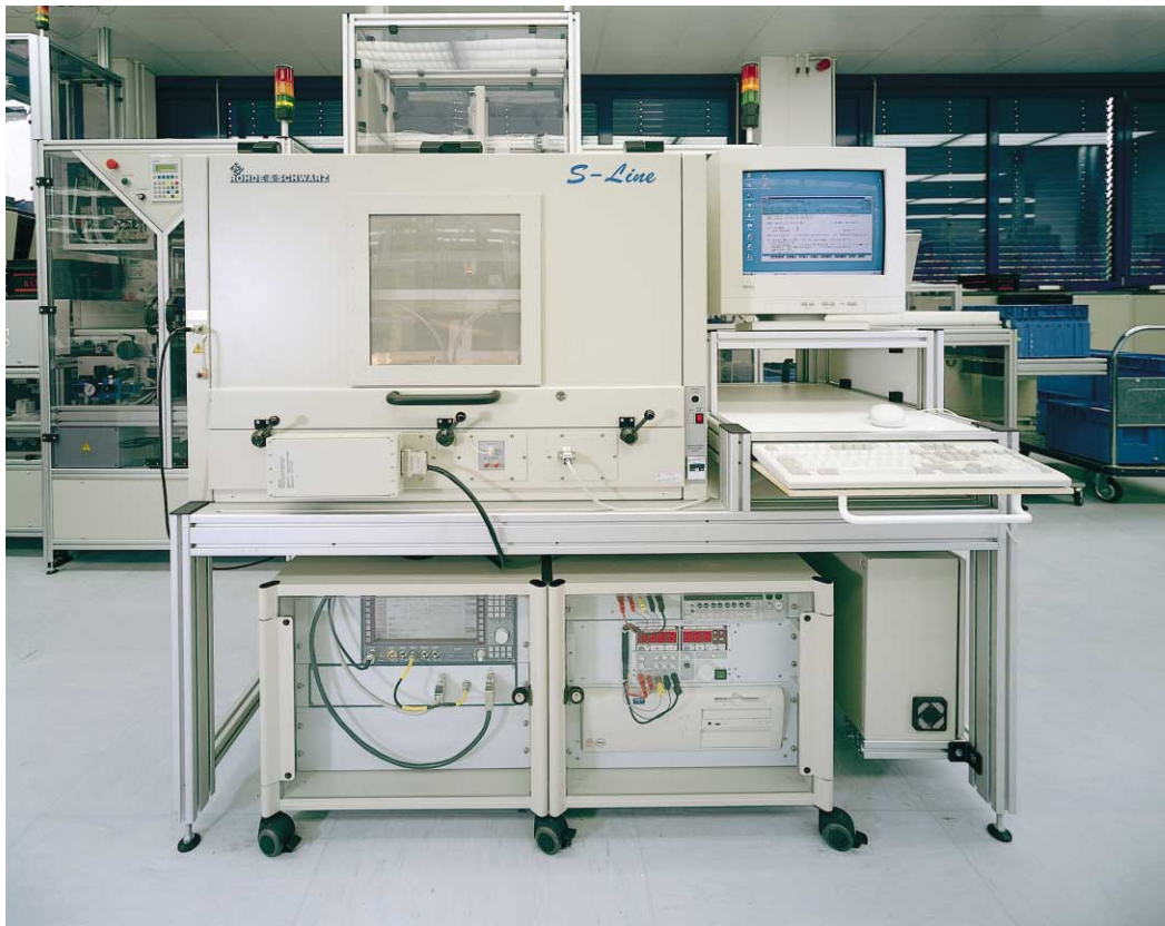
FIG 2 Radiocommunication Service Monitor CMS54 (bottom left) together with Universal Test System TSU used for functional testing of receivers (in EMC Test Cell S-LINE 700/P) Photo 43 027/2
